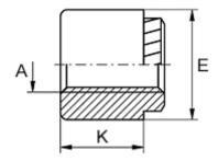
Female thread A = M3 Height K = 5 Hole diameter +0.1 = 4.2 Min distance to edge = 2.4 Min material thickness = 1.5 Outer diameter E = 7
